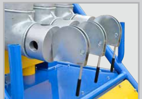
Filter cleaning Controls
