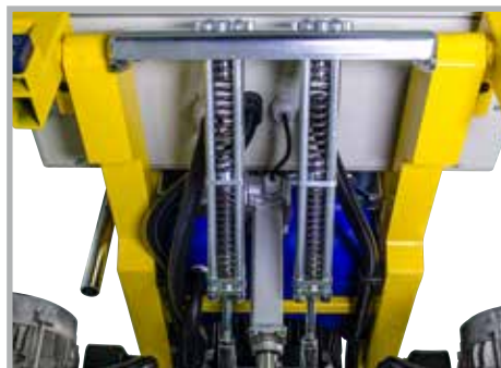
Adjustable working pressure
