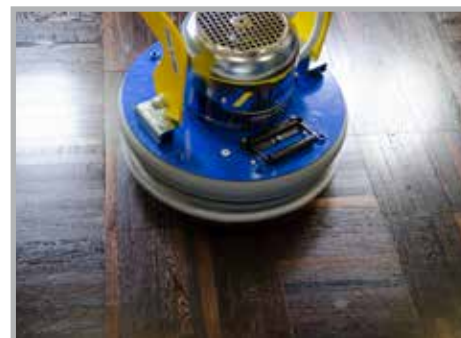
Oil finishing with raised wheels
