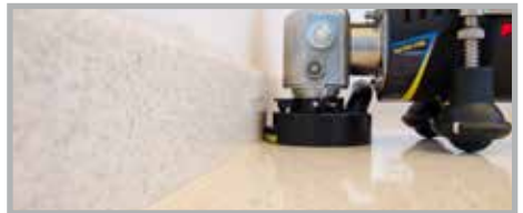
Grinding and polishing perimeters and edges.
