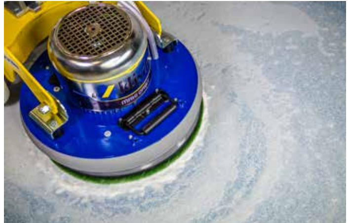
De-waxing linoleum, PVC and rubber
