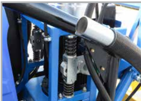
Auto-Levelling Planetary System
